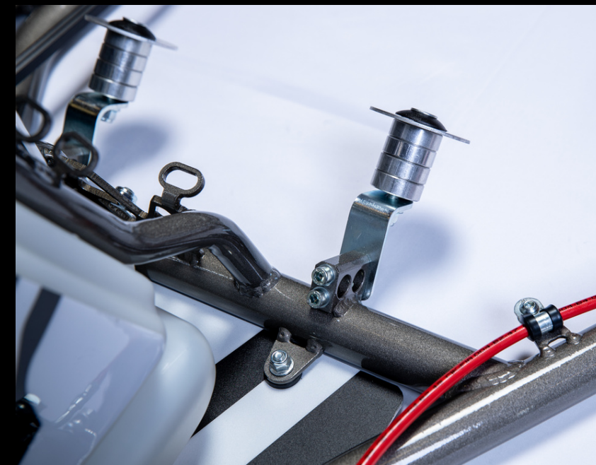
Redesigned bottom and top seat supports. Lower support becoming a bolt on support for easier and more efficient seat installation. Upper support has been reinforced for more durability.
