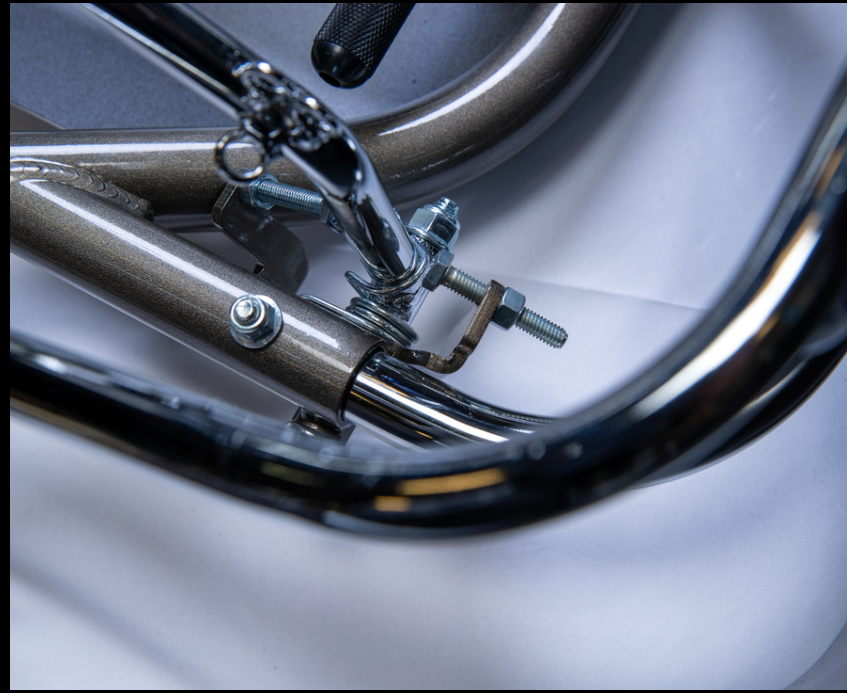
Redesigned pedal mounting system that allows more pedal range along with reducing welding onto the primary tubes of the frame.
