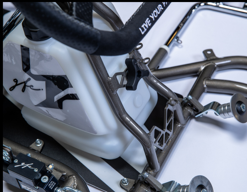
Relocated fuel tank placement to help weight distribution changes during long races.
