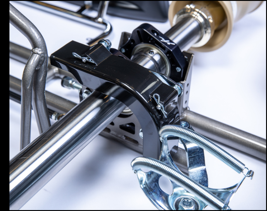
Redesigned chain guard single piece mounting system with quick release pin system.
