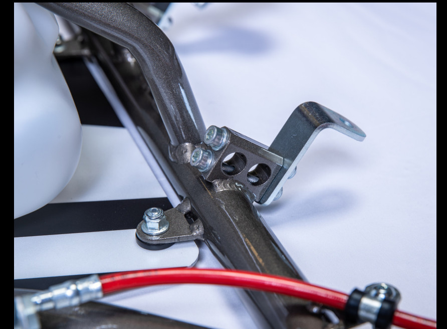
Redesigned bottom and top seat supports. Lower support becoming a bolt on support for easier and more efficient seat installation. Upper support has been reinforced for more durability.
