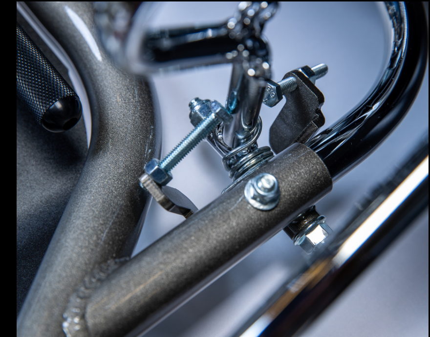
Redesigned pedal mounting system that allows more pedal range along with reducing welding onto the primary tubes of the frame.
