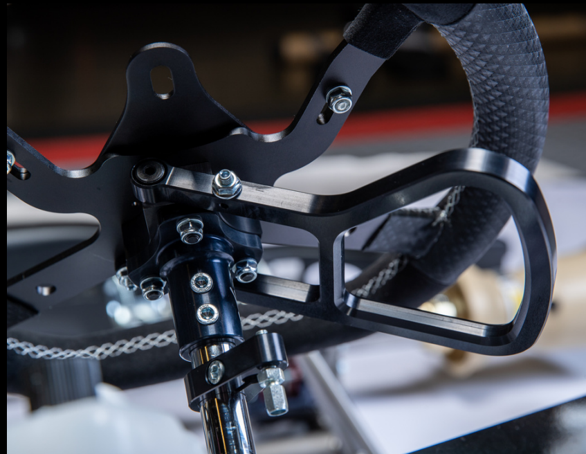
Redesigned clutch lever with smoother feel and greater adjustability.
