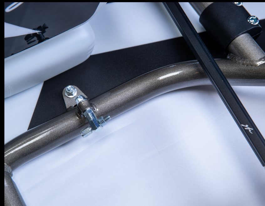
Redesigned throttle cable housing locator to allow more range of adjustability.
