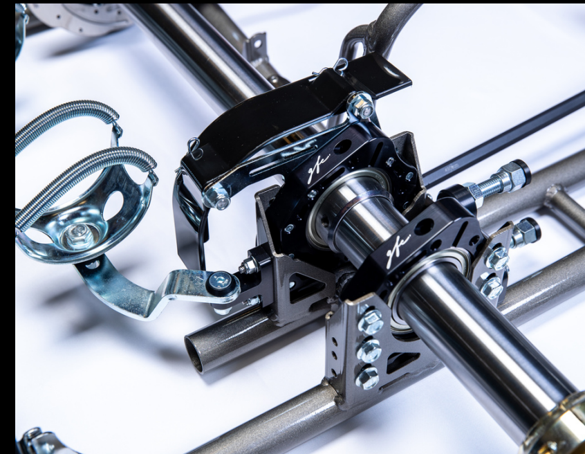
Redesigned rear bearing supports with more rigidity and weight reduction.
