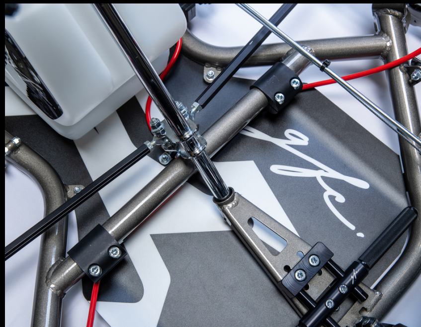
Redesigned steering geometry to give drivers more stability and control upon initial turn in.
