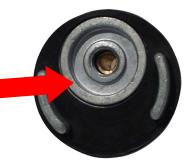
Slide opening must not exceed the appropriate 'no go' specification as per class regulations. For information on slide optimization see video section at <a href="https://www.BriggsRacing.com">www.BriggsRacing.com</a>
